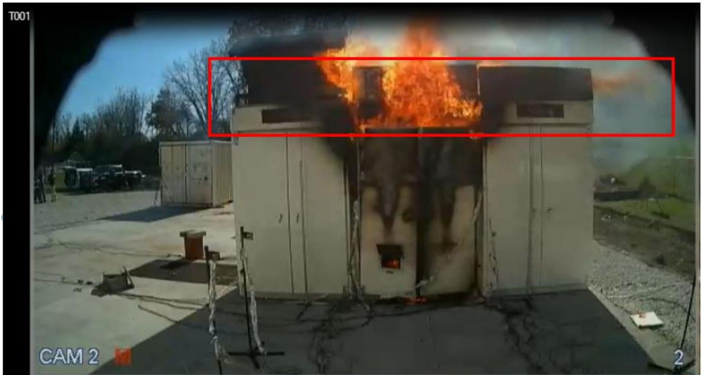
Figure 31: Fire spread through the ladder tray area.
